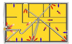
system. The by-pass vent is installed in the same room where the fireplace is located and is connected to a fan with a minimum of 2m of flexible aluminium pipe.
