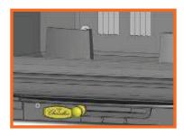
Primary air damper in position 1 and draft shutter closed.
